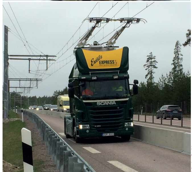
Figure 3: In-road conductive demonstration track at Arlanda, Sweden (upper) and overhead catenary lines demonstration track outside Gävle, Sweden.
