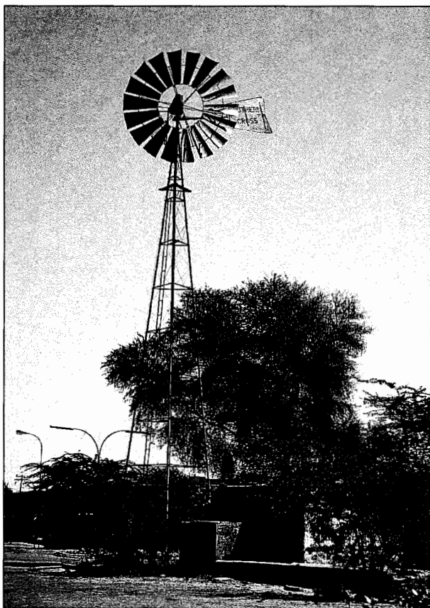
Gear-driven windpump, India.
